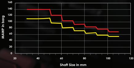
Silicon Carbide vs Silicon Carbide (3600 RPM)
